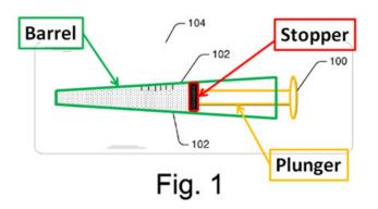
Petitioner's annotated and highlighted Figure 1 of Sigg, with the barrel labeled in green, the plunger labeled in yellow, and the stopper labeled in red. Pet. 41.
